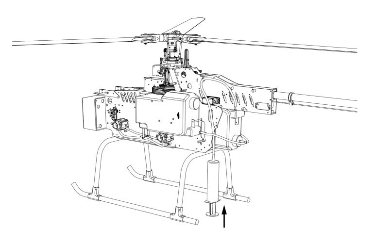
When all fuel tanks are filled with fuel you will need to inject some air back to the fuel pipe to avoid siphon phenomenon.
