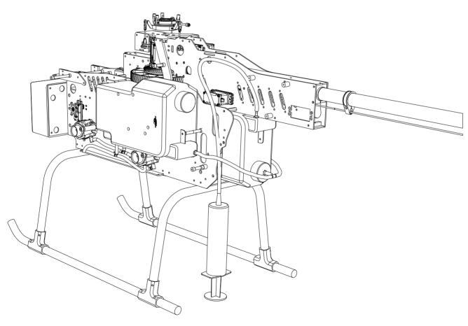
Connect the pipe which is at the end of the main tank to a syringe. When the main tank is full please make that the pipe is well connected to the syringe to avoid leakage of oil, then proceed to fill up the external tanks.
