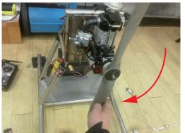
7.Turn the propeller and bring piston out of compression point (makes the motor start easier), turn the switch-on and turn the switch-off when fuel enter carburetor.
