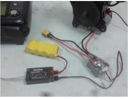
Connect the signal cable to receiver. Connect battery to receiver for testing the switch; please don't connect the main power battery during testing.
