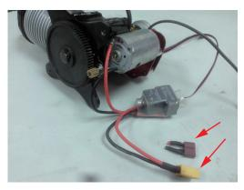
Connect one electric wire to motor from main power switch and one to battery connector. (make sure the connector is correct) There is no in-put/out-put different in these two wires.
