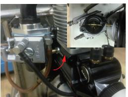
8.Open the air choke, when propellers bring piston leave compression point then open CDI power to get the engine started.
