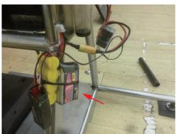
Connect main power battery for start testing. The battery capacity needs to be bigger than 800mAh and using 3S.
